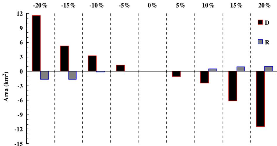
Fig. 13. Sensitivity of the area of high vulnerability of GCA to contamination due to different perturbation percentages in the depth to water table and groundwater recharge.
