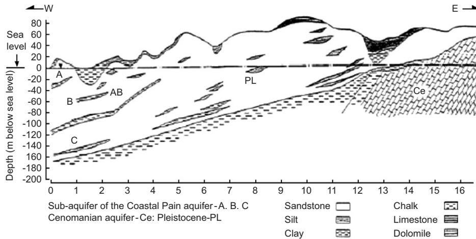
Fig. 4. Generalized geological cross-section of the coastal aquifer (Baalousha, 2003).
