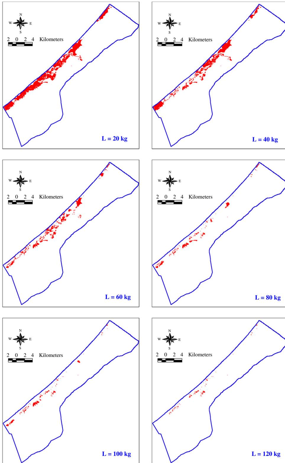
Fig. 15. The spatial distribution of the high vulnerability areas that correspond to the different on-ground nitrogen loading levels ( $L$ ).
