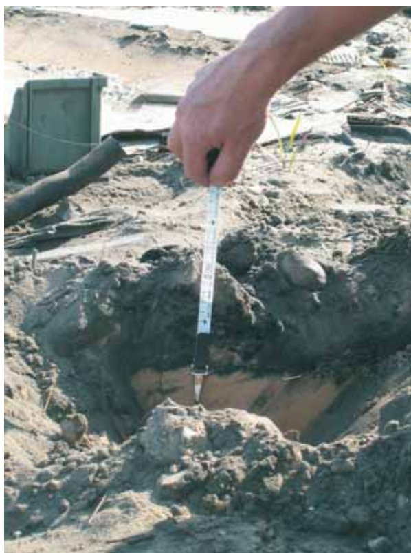
The maximum depth of the impacted "burned" zone at location A was 10 centimeters
