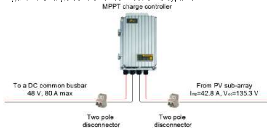
Figure 1. Charge controller connection diagram.
