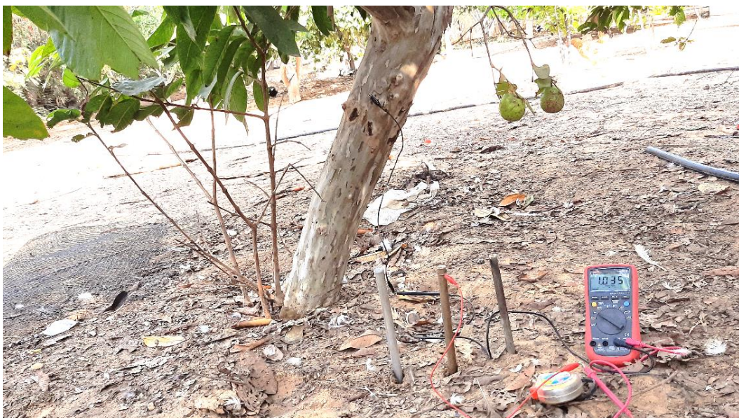
Figure 2: Connection of multi-meter probes to the electrodes (cathode and anode probes are connected to the trunk and ground electrodes, respectively)
