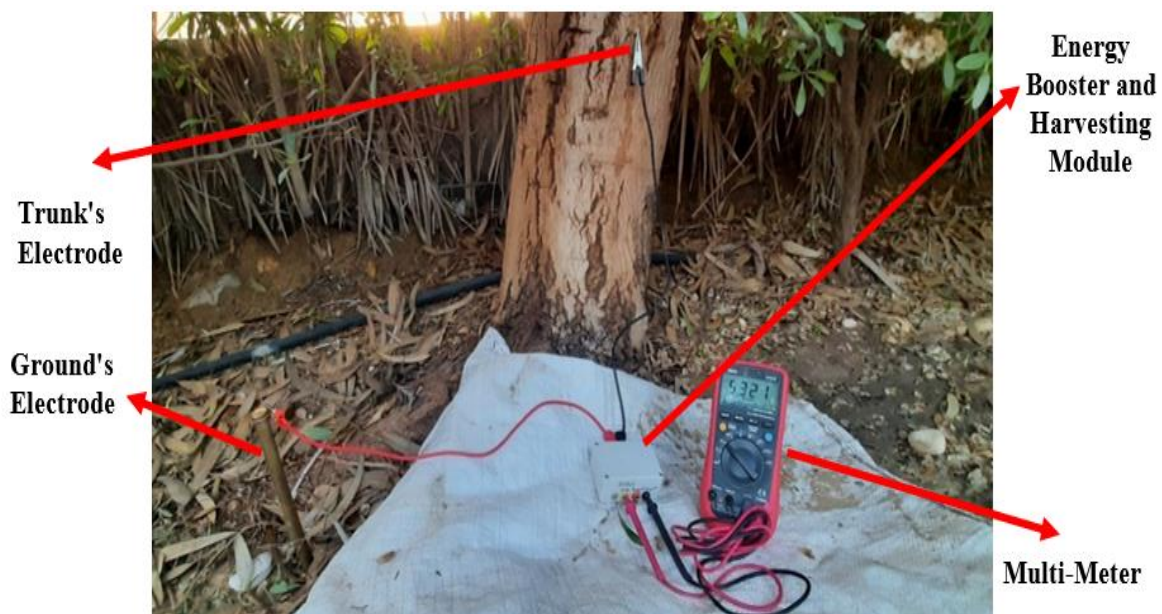
Figure 10: Boosting and harvesting the low voltage energy produced from a Eucalyptus tree to greater than 5V using EH4295 and EH301A modules.
